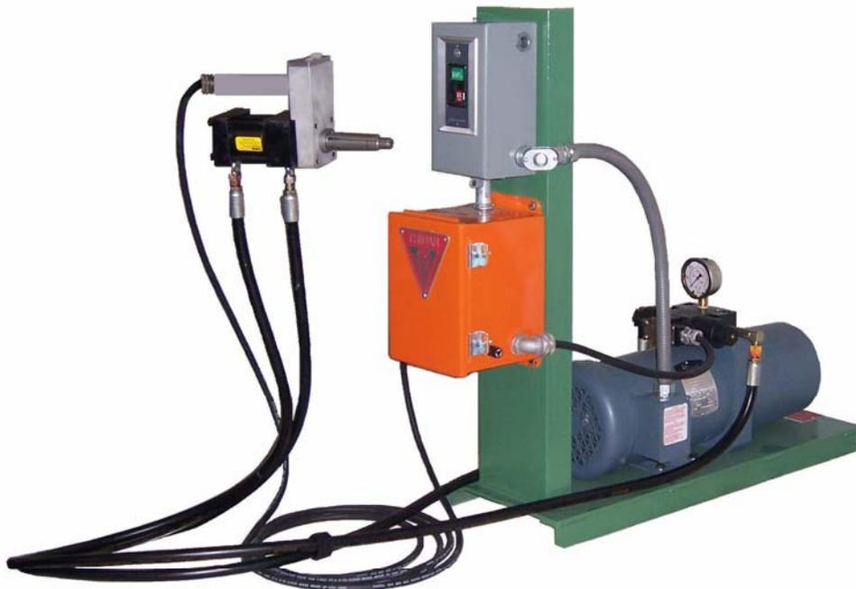
This Tridan **Model BTH Tube End Sizer** is a hydraulically driven device that is specially designed for belling the end of heavy wall tubing. An electrical solenoid valve is used to control the hydraulic operation.
