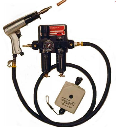
The Model **BFA Tube End Sizer/Flarer** is an air operated vibrating type device that is designed to produce a final bell and flare on the end of a heat transfer coil tube extension. The bell and flare will allow for the insertion and brazing of return bends or other related fittings.
