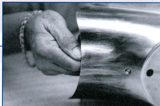
Figure 4-1. With moderate thumb nail pressure, the wiper's leading edge must deflect evenly all around, often 0.005" to 0.010" (0.13 mm to 0.26 mm).
