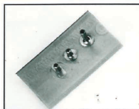
Unusual applications include staking and dowelling. Here, steel studs are welded onto a plastic auto trim.
